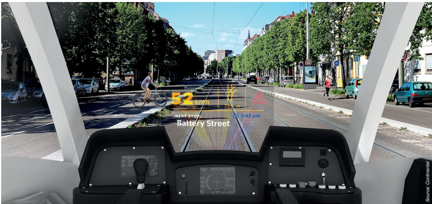
Illustration 1: Example of a Combiner head-up display for driver assistance with selected information, navigation instruction and warning signal
