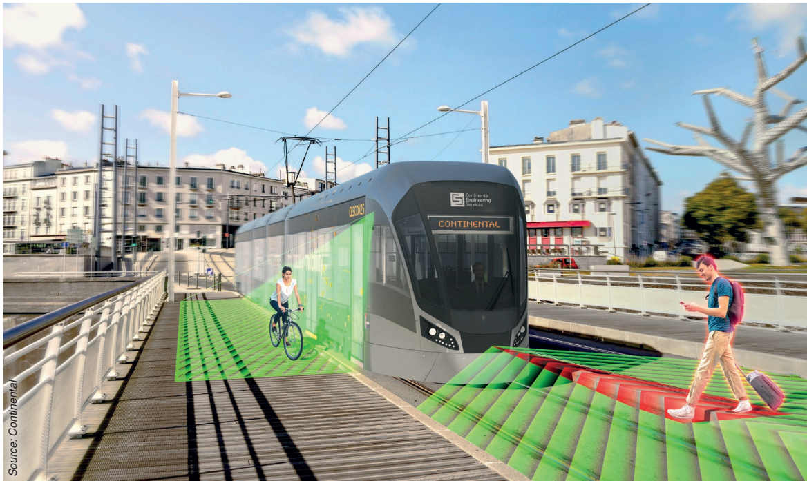
Illustration 5: Monitoring of the driving environment to the side and ahead
