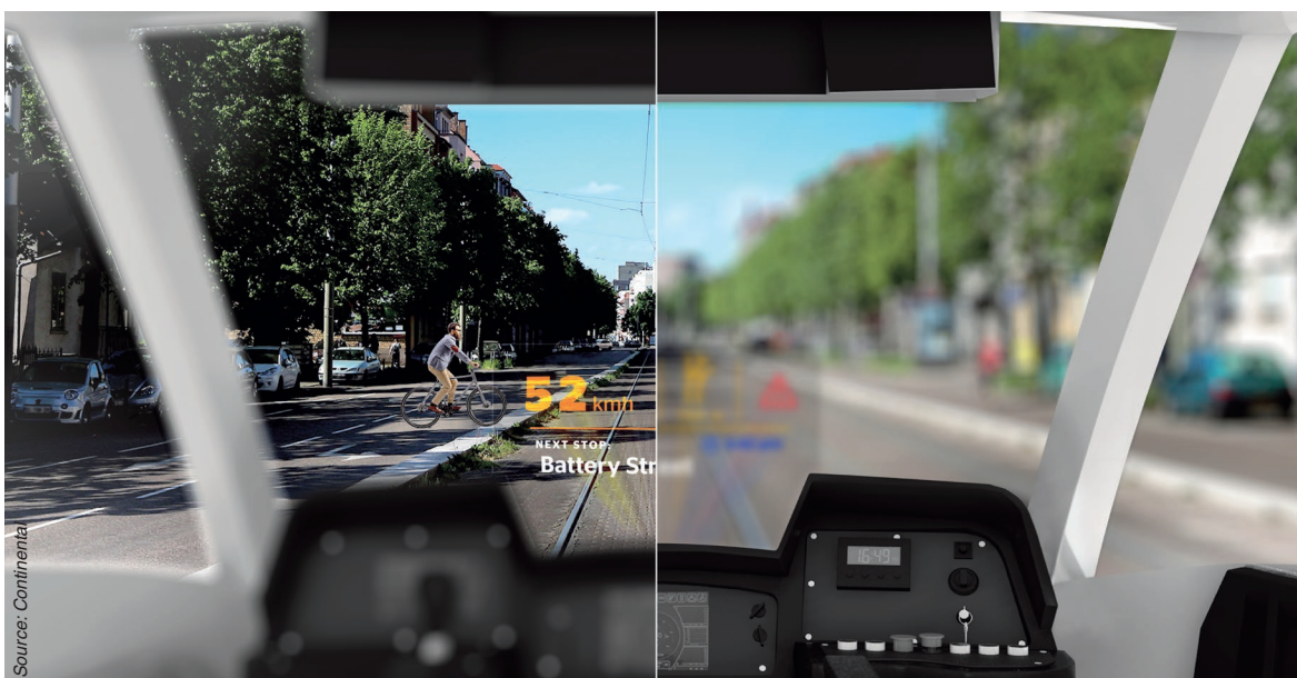
Illustration 3: Effect of a Combiner head-up display: The focus planes of the display and traffic situation are close together (left half of the image), unlike with the conventional instrument (right half of the image)
